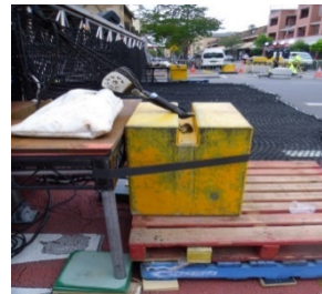
1tonne concrete ballast
